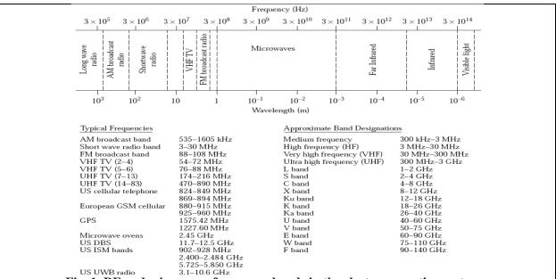
Fig. 1. RF and microwave frequency bands in the electromagnetic spectrum
